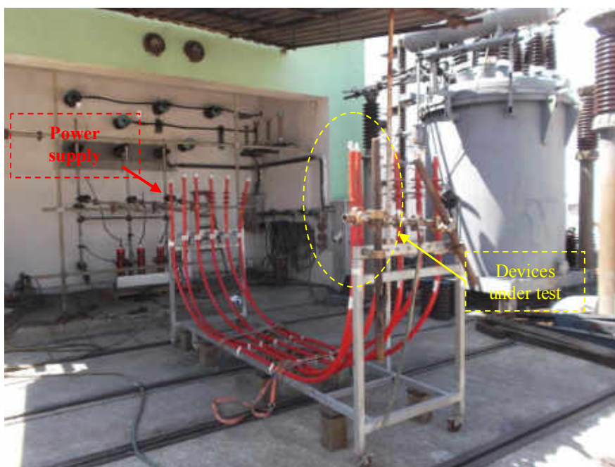
Photo 13: arrangement for thermal short-circuit test on screen/armour
