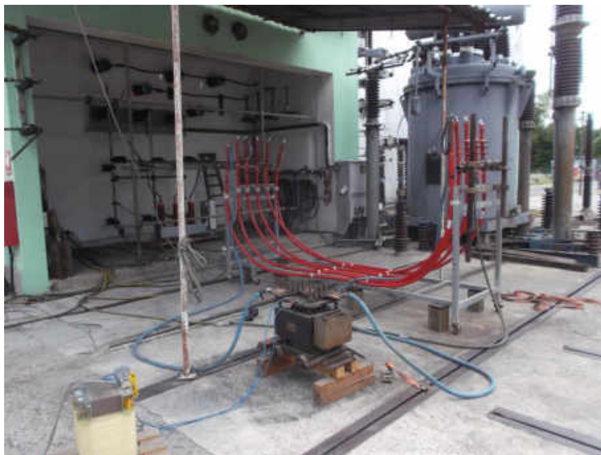
Photo 12: arrangement for heating cables
