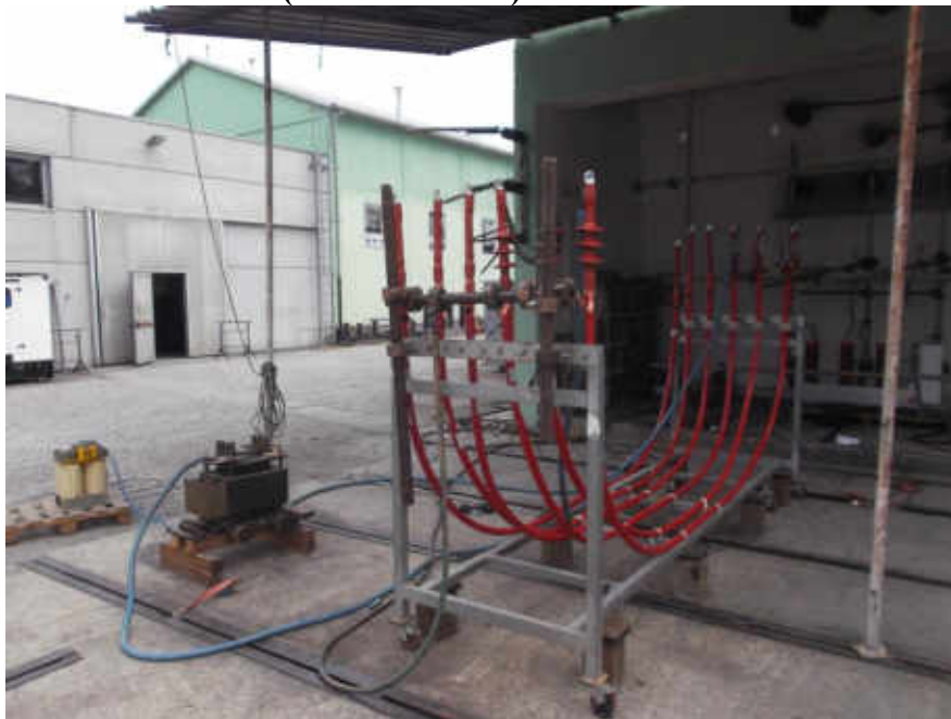
Photo 1: arrangement for heating cables
