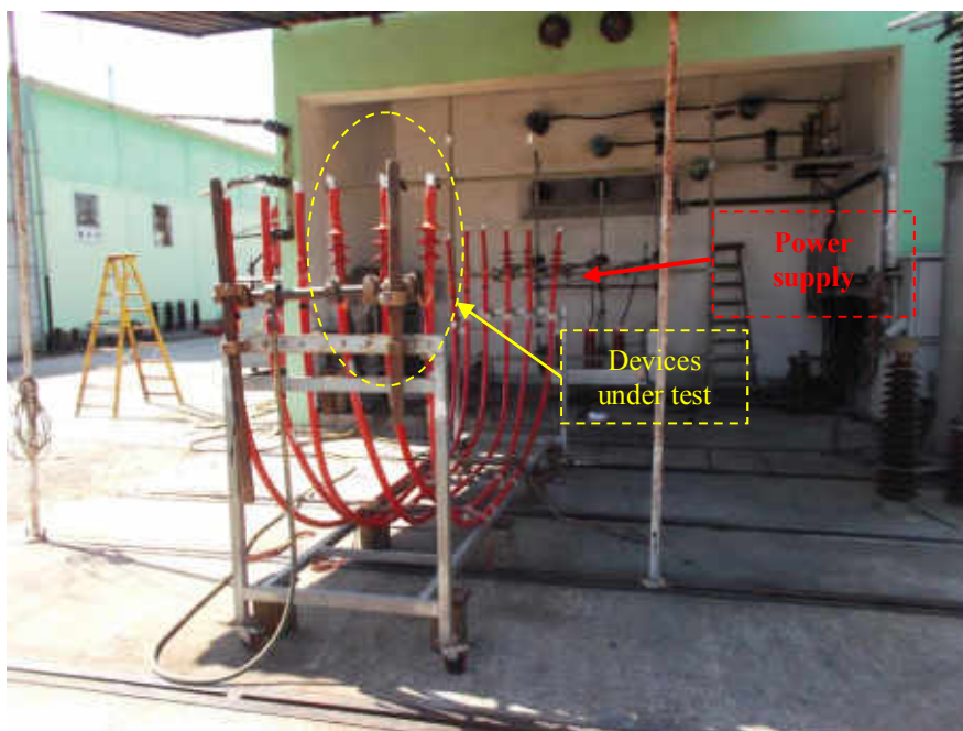
Photo 2: arrangement for thermal short-circuit test on screen/armour
